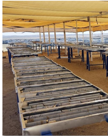
Diamond drill core logging racks at Hawiah.
